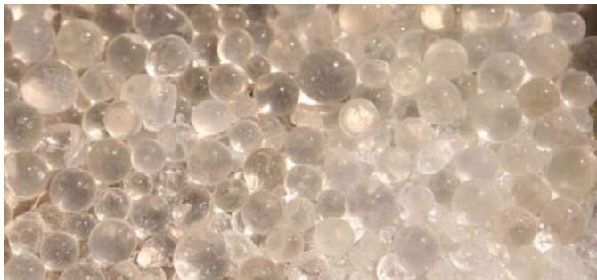
Fig. 4 Drying agent, colorless
